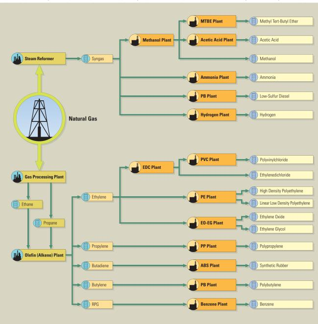
Figure 1: Hydrocarbon processing flow diagram indicating a sampling of manufacturing units that benefit most from process mass spectrometry
